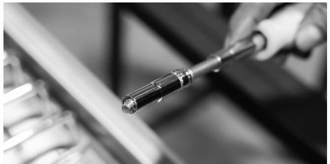
Replace the ORIFICE with the LP ORIFICE that came with your SIDE
