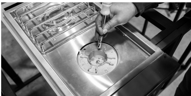
Replace the NG ORIFICE with your LP ORIFICE. Re-tighten.
