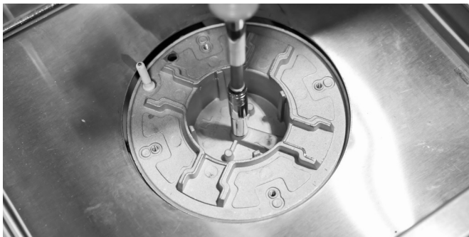
Loosen and remove the NG ORIFICE
