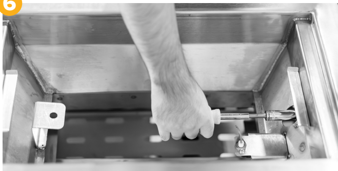
Replace the NG Orifice with your LP Orifice. Then, Re-tighten
