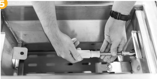
Use a 13mm socket to remove the NG orifice
