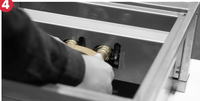
Gently pull and lift the Burner
