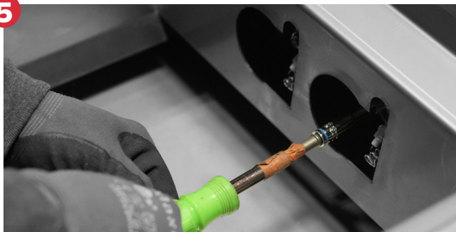
Use a 6mm socket to remove the NG orifice
